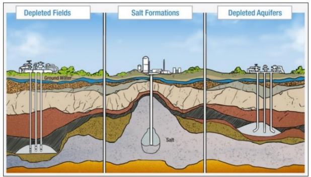
Figure 1: Underground natural gas storage (API, 2016)
